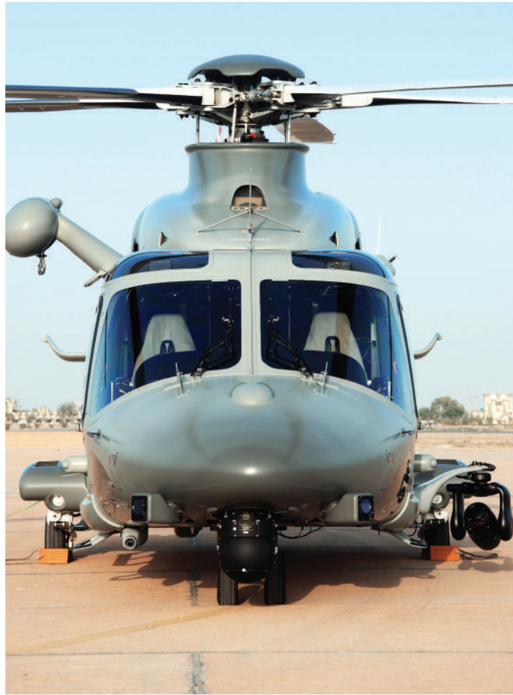
▲ The AW-139 Seahawk has a Breeze-Eastern hoist on the starboard side, a FLIR under the nose and a Trakker searchlight on the port side
