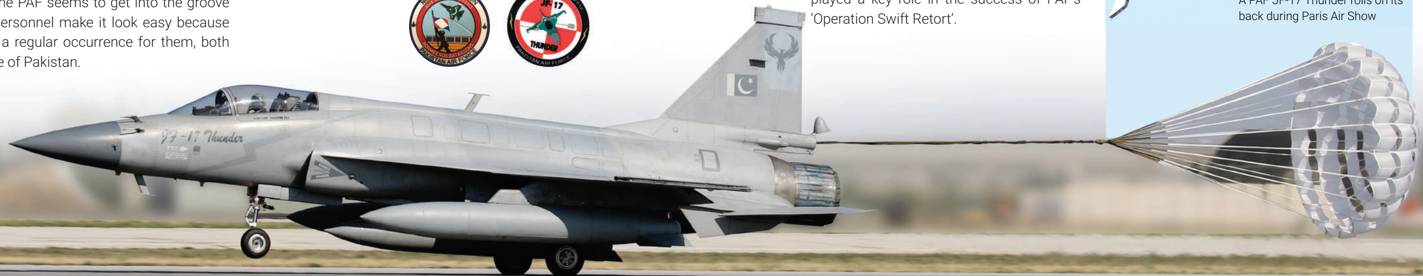
A fully extended chute breaks the speed of a JF-17, as the pilot lowers the nose wheel on landing
