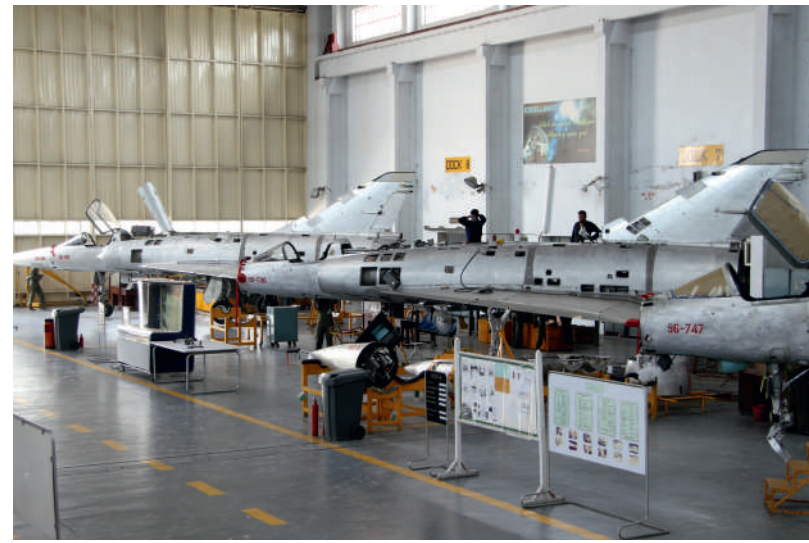
Mirage Rebuild Factory (MRF) in PAC Kamra has played a key role in maintaining the Mirage fleet for more than five decades. A routine view from a jet shop of MRF shows the Mirage aircraft being overhauled by the team of professional technicians. (Photo : PAF Archive)
