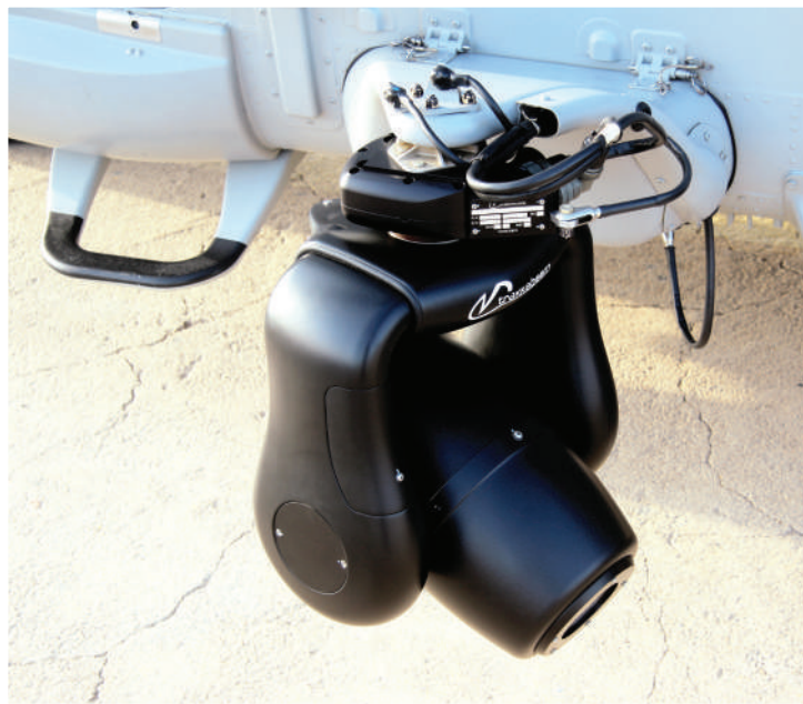
The Trakker searchlight will provide the aircrew with a strong enough light to understand the working conditions ▼
