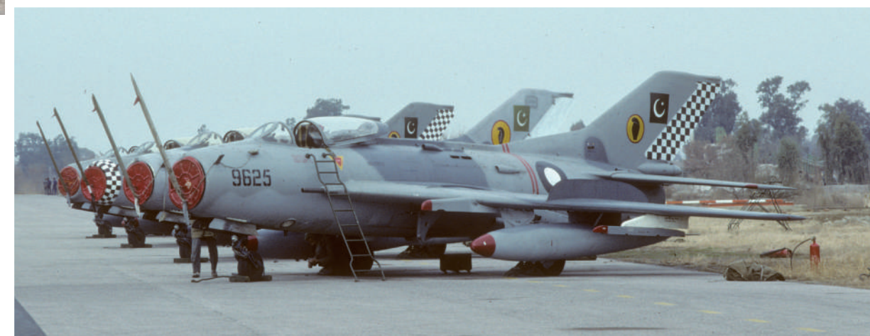
Left Page Bottom: F6 matures into a capable weapon system- PAF made significant modifications to its F-6 fleet, most notable being AIM-9B Side winder. (Photo: Peter Foster)
