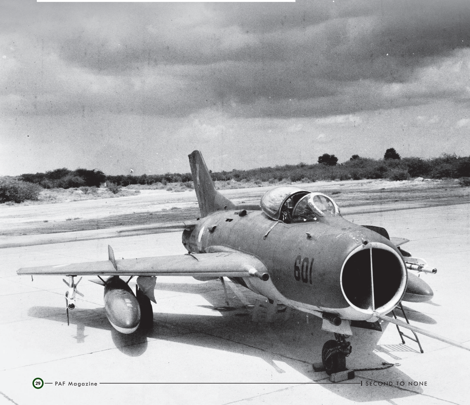
Bottom: Twin - engine monster armed with AIM-9B remained a potent aircraft for decades. (Photo: PAF Archives)
