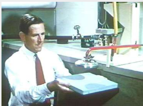
"Jack" Frost demonstrates the Coandă effect. Pressurized air flows out of the end of the red tube, and then over the top of the metal disk. The Coandă effect makes the air "stick" to the disk, bending down at the edges to flow vertically. This airflow supports the disk in the air. (Photo: blogto.com).
