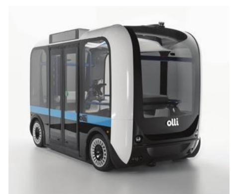
Local Motors' Olli is a 3D printed shuttle made by using 90% fewer parts than its assembly-line produced counterpart. (Photo: Local Motors).
