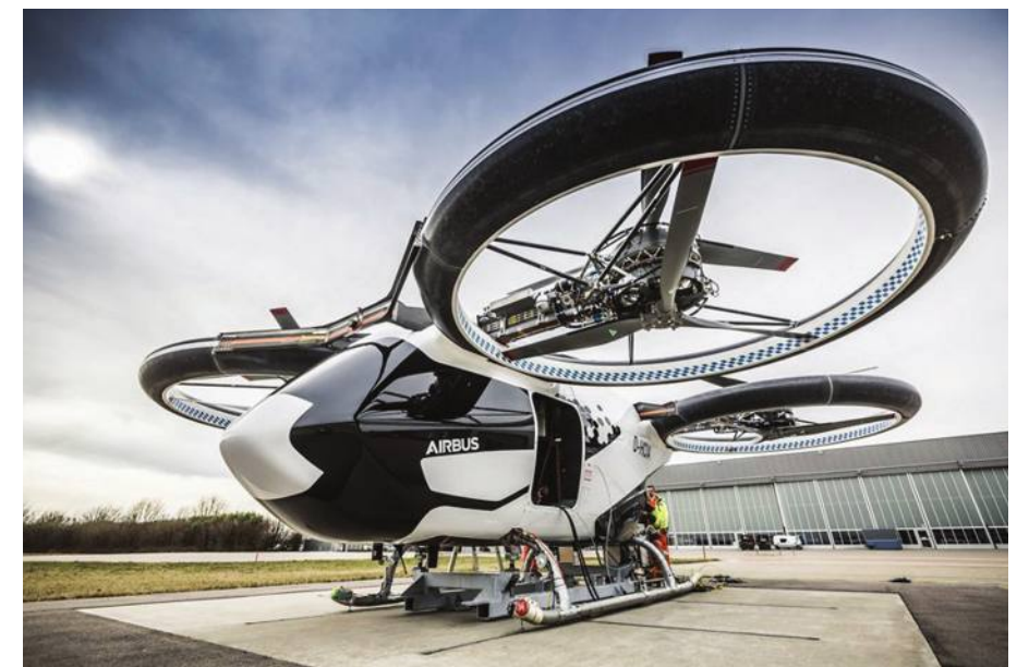
CityAirbus is an all-electric, four-seat, multicopter vehicle demonstrator that focuses on advancing remotely piloted electric vertical take-off and landing (eVTOL) flight. (Photo: Airbus).
