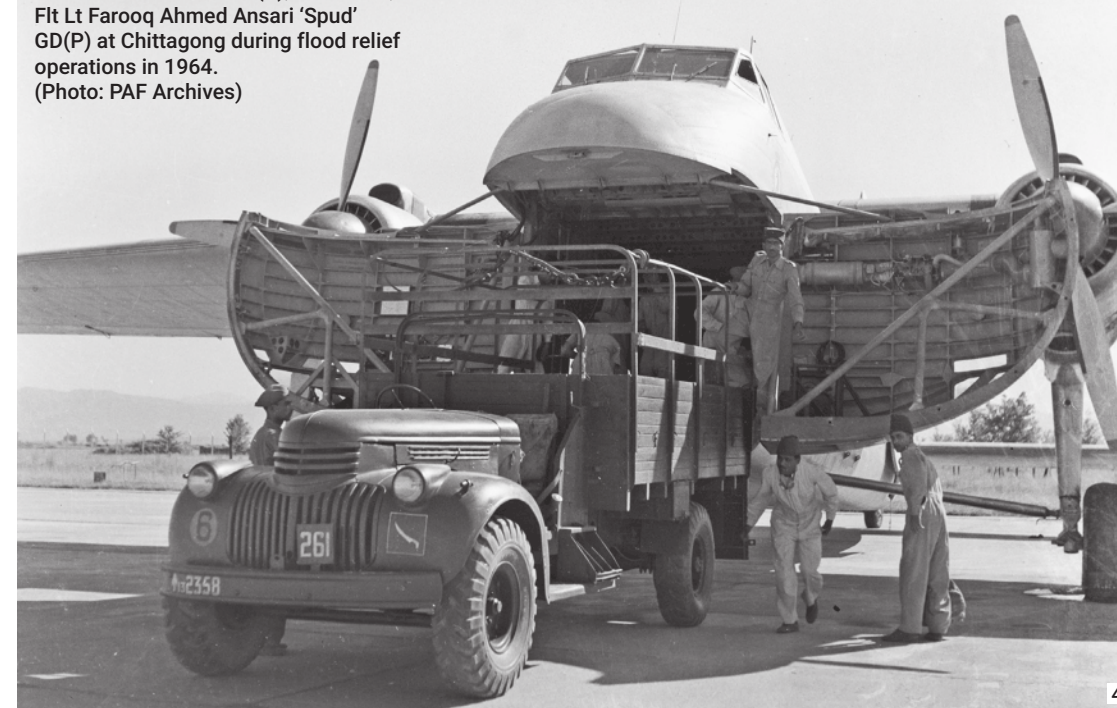
4: No 12 Sqn's Freighter ready to be offloaded at Chittagong during relief flood operation in July 1964. The advantage of clamshell door is clearly visible, allowing to move the freight directly onto a lorry. (Photo: PAF Archives).
