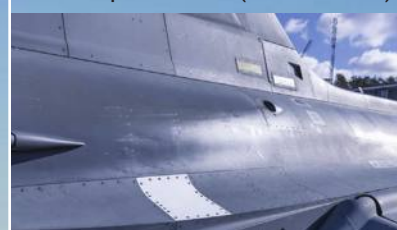
The inlet shows the closer view of the 3D printed hatch. (Photo: Saab AB).
