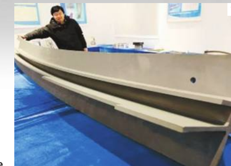
1: Central wing flange 3D printed in titanium for the Comac C919. (Photo: 3dprintingindustry.com).
