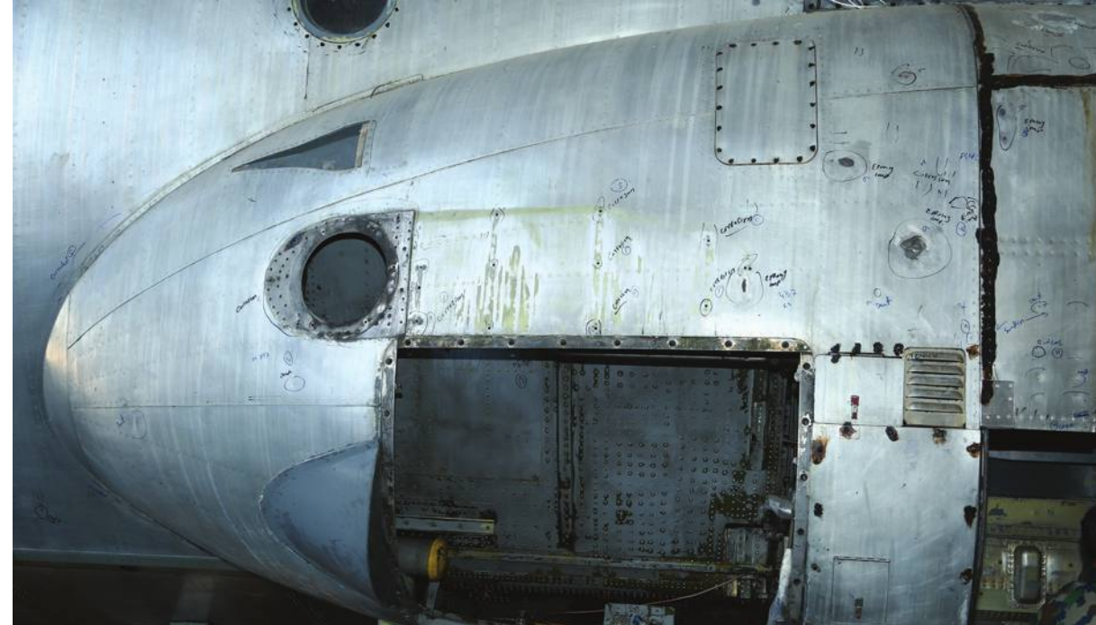
Left: Inspection crews circle signs of wear with blue marker, centimeter by centimeter.
